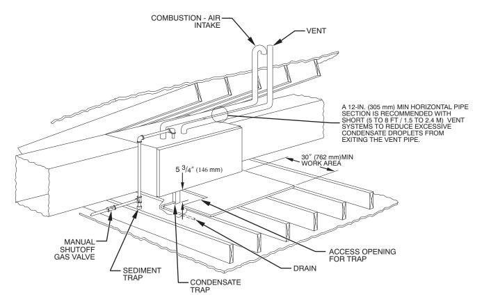
NOTE: LOCAL CODES MAY REQUIRE A DRAIN PAN UNDER THE FURNACE AND CONDENSATE TRAP WHEN A CONDENSING FURNACE IS INSTALLED ABOVE FINISHED CEILINGS.
